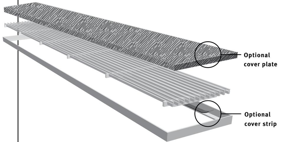
When the trench is installed in a concrete floor, the wooden spacers or optional cover plate must be installed before the concrete is poured. This will prevent deformation of the trench.
