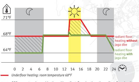
DBE convectors in combination with radiant floor heating: the radiant floor heating provides a base temperature of 64°F, while the responsive DBE radiators ensure a perfectly regulated and stable comfort temperature of 68°F. With this combination, energy savings of 33% are achieved! Test conducted in the Jaga Experience Lab (www.heating-studies.org)
